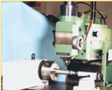
TAWN 160 NEGi 4th axis mounted on a vertical machining centre control via M-function
